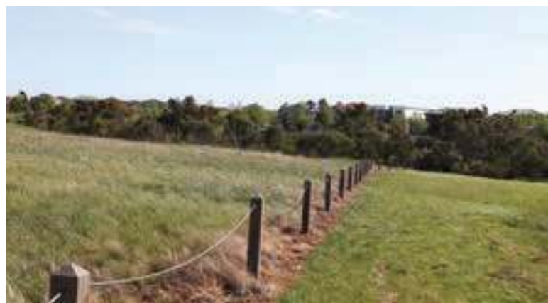
Steel cable fencing is visually unobtrusive, not uninviting, and is effective at preventing vehicle entry. Shown here, Isabella Williams Memorial Reserve, Albanvale.
