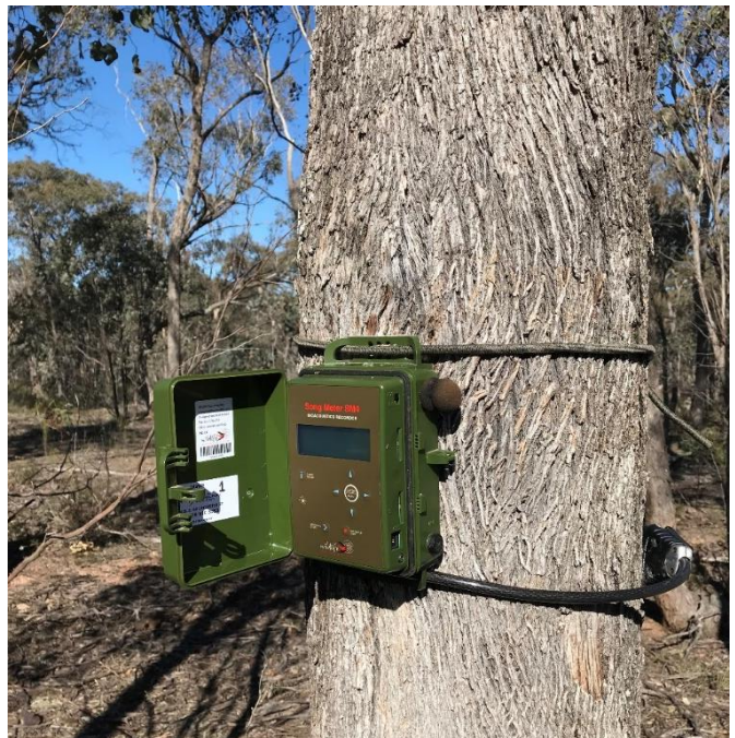
Song Meter SM4 acoustic recording device. Photo: Sera Blair
